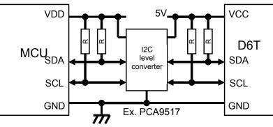
Fig. 9. Using a Level Converter
