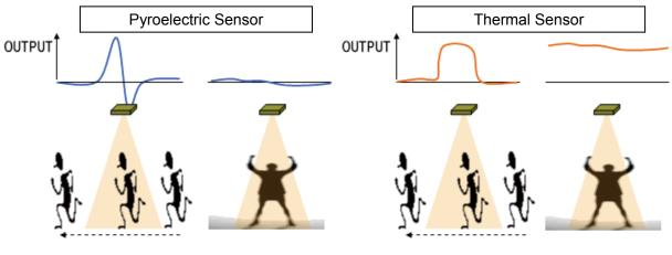
(a) Output of pyroelectric sensor
