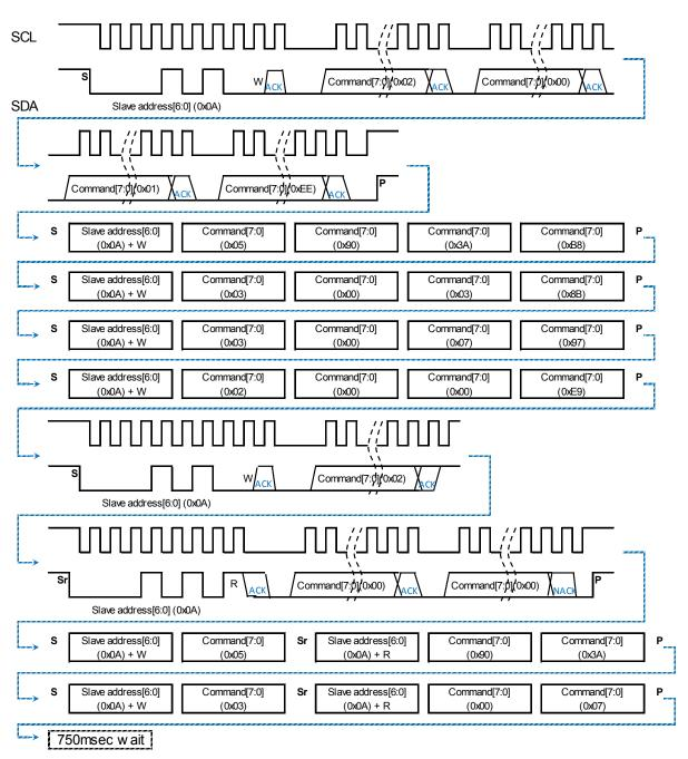
Fig. 17. Signal Terminal Flow (D6T-8L-09)
