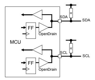
Fig. 10. Using a GPIO Terminal
