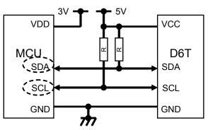
Fig. 8. 5 V Fault Tolerant Specification
