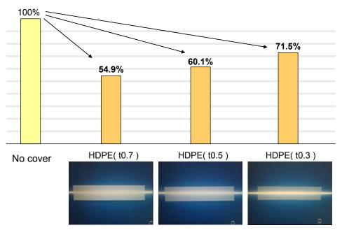
Fig. 23. Relationship Between HDPE Thickness and Transparency (Reference)
