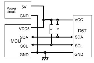
Scenario 1: 5 V MCU Direct Connection (Same voltage as the microcontroller power supply)
